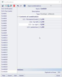
It is also possible to explode this combination to view all the linear combinations it holds. If you do this, Combi26 – 31 will be created. This time the user defined partial factors are used. This combination also makes sure LC2 and LC3 never occur together because their relation was set as 'exclusive'.
